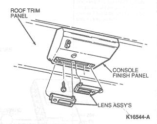
Install the map lamp lens assembly by engaging lens retaining tab at outboard edge of opening and snapping center edge of lens into console.
