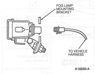
3. Slide fog lamp out of mounting bracket assembly.
