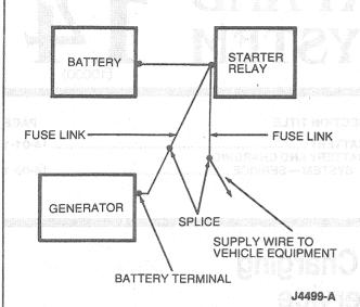
Service fuse links are brown, green or black depending on usage. All fuse links have a flag moulded on the wire or on the terminal insulator. Color identification of the flag or connector for the external voltage regulator system is brown 18-gauge wire or gray 12-gauge wire. The illustration shows a typical fuse link installation.
