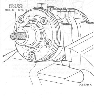
17. Using Shaft Seal Remover/Replacer
