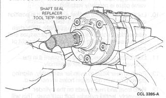
Attach shaft seal seat to Shaft Seal Seat
