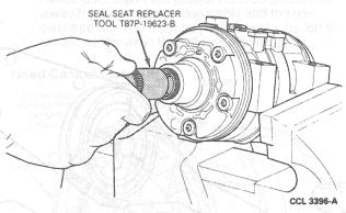
Install seal seat retaining snap ring into nose of compressor and push snap ring into the groove with handle end of Shaft Seal Remover / Replacer T87P-19623-C.
