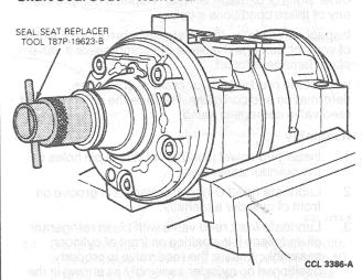
Insert Shaft Seal Remover / Replacer T87P-19623-C into compressor nose opening and on top of shaft seal. Rotate tool clockwise while pushing tool inward until tool engages tangs of seal. Then pull shaft seal from compressor with tool.
