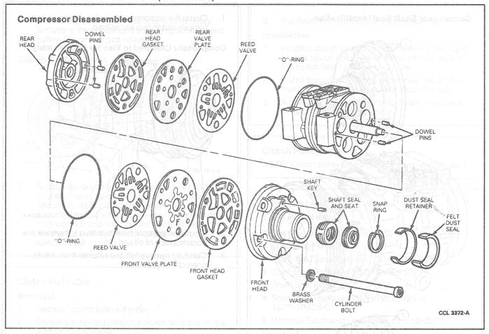
Remove shaft key with Shaft Key Remover T81P-19623-NH.
