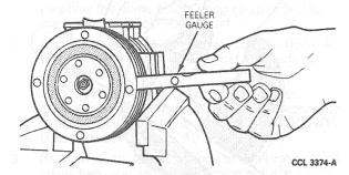
Rotate compressor pulley one-half turn (180 degrees) and again check air gap in three equally spaced locations. Smallest air gap must be within specified limits for air gap. Add or remove shims between hub and compressor shaft end as necessary until smallest air gap is within specification.
