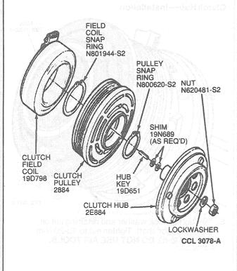
3. Pull field coil from front of the compressor.
