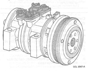
Reed-type suction and discharge valve plates are located between the cylinder assembly and the head at each end of the compressor. The heads are connected with each other by gas-tight passageways which direct refrigerant gas to a common output.
