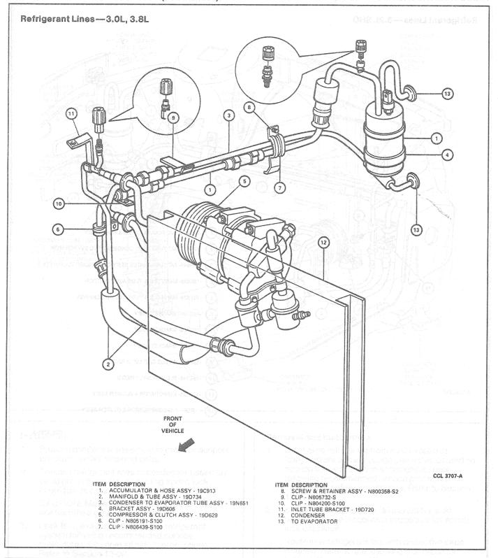
4. Connect refrigerant line into system using new O-rings lubricated with clean specified refrigerant oil. At condenser, use connecting procedure for spring lock couplings.
