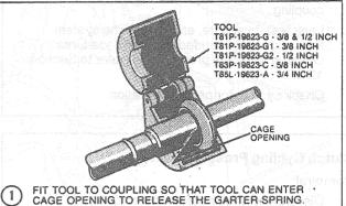
**PUSH TOOL INTO** CAGE OPENING PUSH THE TOOL INTO THE CAGE
