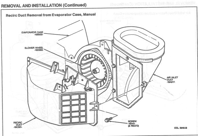
Remove two screws from air inlet duct and remove duct from evaporator case.
