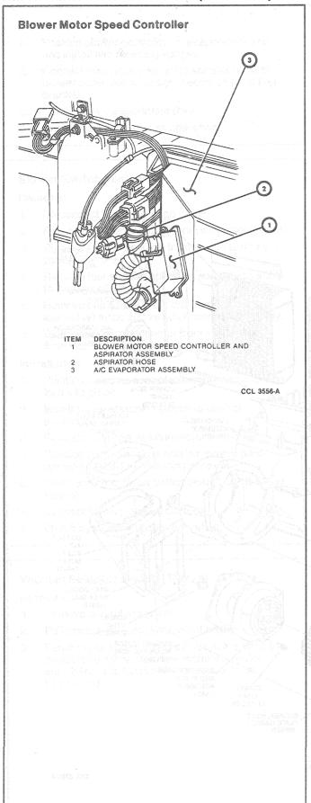
3. Remove two screws retaining blower controller to evaporator case and remove controller. Do not touch fins of controller until it has had sufficient time to cool.
