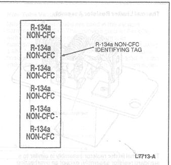
If the A/C system has any of the R-134a identifying characteristics outlined, R-134a refrigerant is the only type of refrigerant that can be used in the A/C system. If the A/C system is not identified as an R-134a system as previously outlined, it is an R-12 system requiring the use of R-12 refrigerant.
