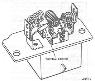
The thermal limiter resistor assembly is similar to a standard resistor assembly, except an overheating protective device (thermal limiter) has been added to prevent heat damage to the evaporator case assembly. Overheating of the resistor coil(s) will occur when the system airflow is stopped as a result of the blower wheel being locked.
