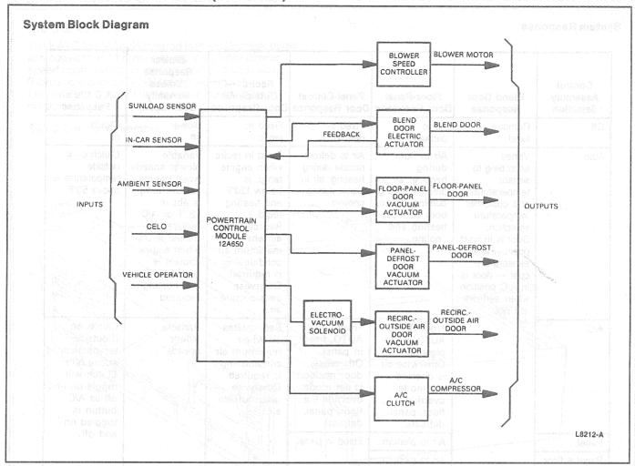
With the use of a microcomputer, the control assembly analyzes inputs from six major sources:
