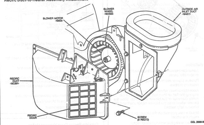
Remove recirc duct from heater assembly, lowering recirc duct from between instrument panel and heater case.
