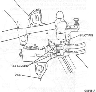
Place two nuts or spacers to hold tilt lock arms away from housing.
