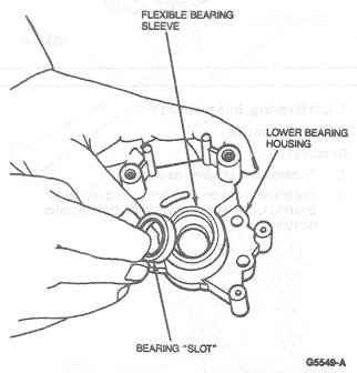
Press in the new bearing with thumb pressure until seated. Slot between inner and outer races should face down when installed in the vehicle.
