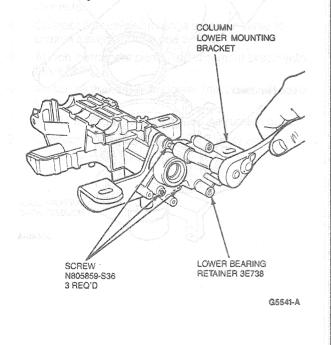
2. Suitably support housing and tap out bearing with a hammer and a drift.
