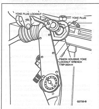
7. Loosen yoke plug with a 3/4-inch socket wrench.
