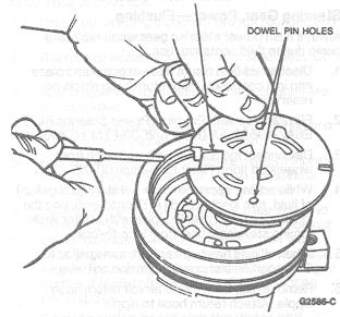
15. Place a new O-ring seal on valve cover. Lubricate this seal with specified power steering fluid.
