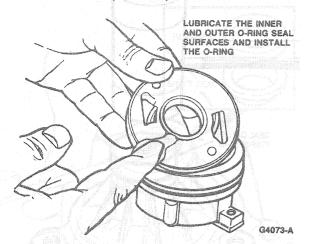
Insert lower pressure plate with O-ring seals toward front of pump into housing and over dowel pins.
