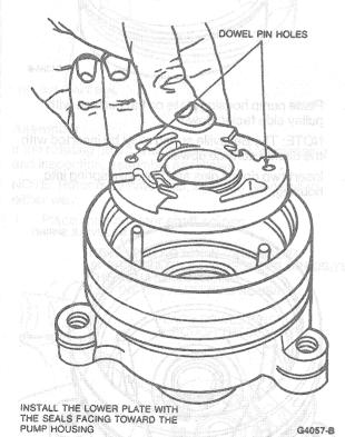
12. Place entire assembly on C-Frame and Clamp Assembly T74P-30441-A1. Place Seal Driver T78P-3733-A3 into rotor shaft hole. Press on lower plate lightly until it is felt to bottom into pump housing. This operation will seat outer O-ring seal.
