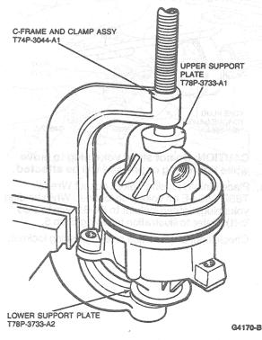
Tighten C-clamp until slight bottoming of valve cover is felt.
