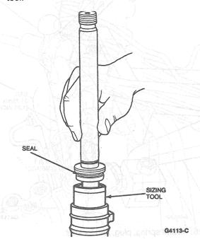
14. Seat rack seal with rack by driving end of rack with a drift or brass bar stock and plastic mallet. Several hits may be required to ensure proper seating. DO NOT remove rack.
