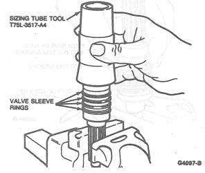
Remove sizing tube, and check condition of rings. Ensure that rings turn freely in grooves.
