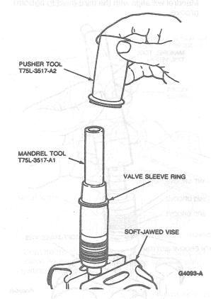
8. Repeat Step 7 using one spacer for second valve sleeve ring (Spacer T75L-3517-A3).
