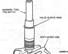
Complete installation by pushing ring into bottom groove.
