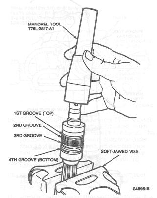
NOTE: Seal grooves do not have port holes. Ensure seals are installed in proper grooves.
