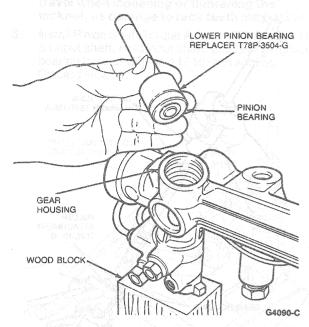
Seat bearing against shoulder in bore. Support valve housing with a wood block when seating pinion bearing.
