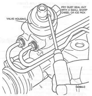
8. Using Retaining Ring Pliers D79L-7000-A or equivalent, remove retaining snap ring, located under dust seal from valve housing.
