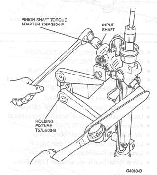
CAUTION: Use care not to damage any valve housing surfaces.
