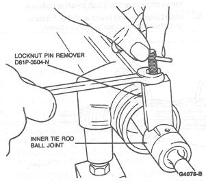
With a sharp chisel, gently tap around rivet head so it lifts away from ball joint. Use caution so the center pin is not sheared off.
