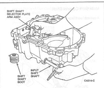
Install the control selector plate. Using a 10mm socket wrench, tighten the retaining bolts to 8-11 N·m (6-8 lb-ft) (pin in selector arm must ride in cutout of gate in the selector plate).
