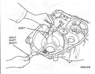
NOTE: Be sure notches in the shift shaft face the detent plunger.
