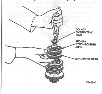
NOTE: When installing the synchronizer, align the three grooves in the fourth gear blocker ring with the synchronizer inserts. This allows the synchronizer assembly to seat properly in the blocker ring.
