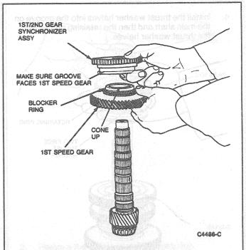
Install the tagged second speed blocker ring and the second speed gear.
