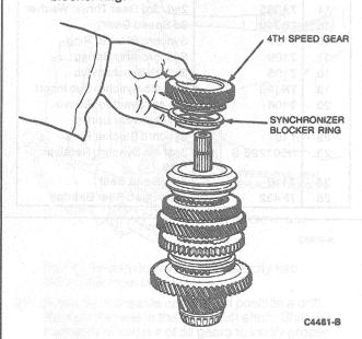
NOTE: Tag blocker ring for proper installation.
