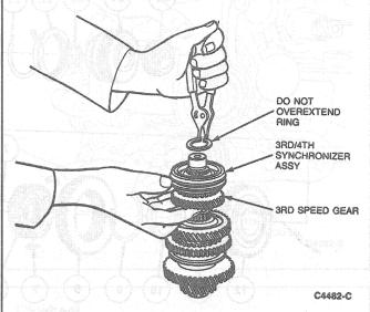
Remove the second/third thrust washer retaining ring and the two-piece thrust washer.
