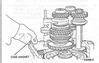
Install the fifth shift relay lever onto the reverse idler shaft, aligning it with the fork interlock sleeve and fifth gear fork slot and install the retaining ring (C-clip).
