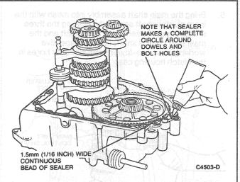
13. Install the detent spring and plunger in their bore in the case. Carefully lower the transaxle case over the clutch housing, then using a punch, depress the spring and plunger.
