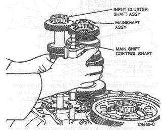
6. Position the shift lever, 3/4 bias spring and fifth/reverse kickdown spring in their working positions (with one shift lever ball located in the socket of the input shift gate selector plate arm assembly and the other in the socket of the main shift control shaft block).
