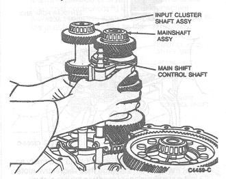
NOTE: Be careful not to drop bearings or gears (slip fit).
