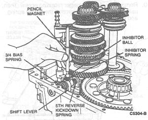
NOTE: Be careful not to drop bearings or gears (slip fit).
