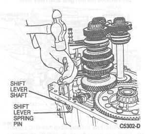
CAUTION: Be careful not to damage main shaft gear teeth or pedestal when prying with the screwdriver.
