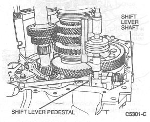
Hold a cloth over the hole in the lever to prevent the ball and spring from shooting out and remove the shift lever shaft.
