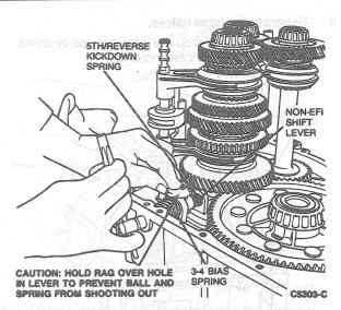
17. Remove the inhibitor ball and spring from the hole in the shift lever using a pencil magnet. Remove the shift lever, fifth/reverse kickdown spring, and 3/4 bias spring.
