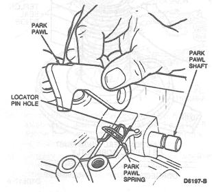
47. Install park rod actuating lever and park rod in case. Install park rod abutment and start abutment bolts. Push in park pawl and locate rod between pawl and abutment.
