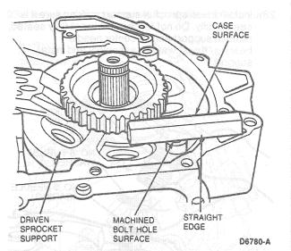
39. If support machined bolt hole surfaces are above case machined surface, place depth micrometer on support bolt hole surface and measure down to case-machined surface. Do this on both holes to get an average. Compare this reading to the No. 8 thrust washer reading in Step 32. The difference between the two readings is the No. 5 thrust washer clearance.
