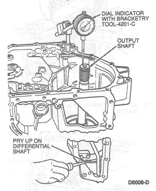
The clearance should be 0.1-0.40mm (0.004-0.016 inch). If the clearance is not within specification, selective thrust washers are available in the following thicknesses:
