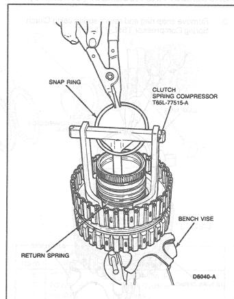
5. Install clutch pack, pressure plate and snap ring into cylinder.
