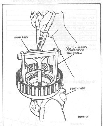
Install wave spring (all except 3.2L SHO), clutch pack, pressure plate and snap ring.
