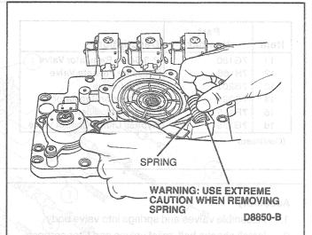
5. Remove outside vane support retaining pin.
