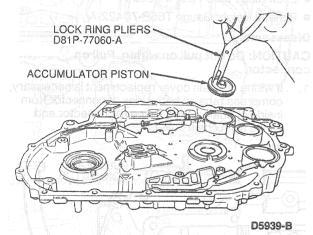
CAUTION: Use care not to damage machined case surfaces or bimetallic strips.
