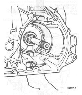
59. Lift out final drive assembly using output shaft.
