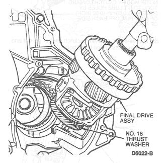
NOTE: No. 18 thrust washer may remain on the final drive assembly next to speedometer drive gear.
