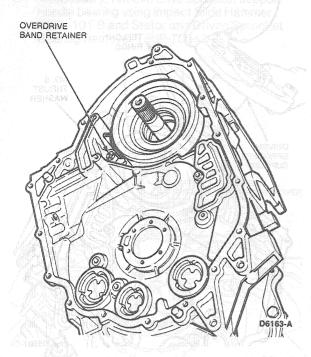
41. Remove overdrive band. Remove screen filter and clean with compressed air.
