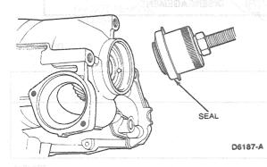
11. Remove two 8mm MLP sensor retaining bolts and remove switch.
