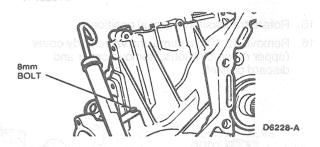
13. Remove five 10mm and four 8mm chain cover bolts from inside torque converter housing.
