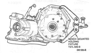
Turn transaxle in vertical position. Remove shipping plugs and drain fluid.
