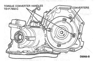
Mount transaxle in Bench Mounted Holding Fixture T57L-500-B.
