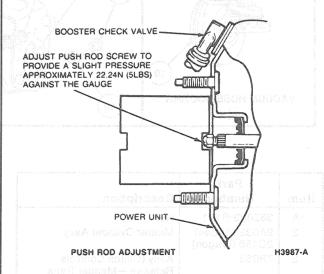
Install master cylinder on booster unit. Gradually and alternately tighten retaining nuts to 21-29 N-m (16-21 lb-ft). Refer to Section 06-00.
