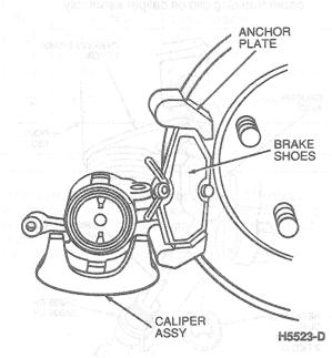
Remove inner and outer shoe and lining assemblies from anchor plate.
