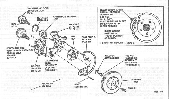
The inner shoes are interchangeable left to right and use a three-finger clip that fits inside the caliper piston. The outer shoes are not interchangeable and use a dual-purpose clip which holds the brake shoes on the caliper housing and also prevents caliper rattle. The flanges on both inner and outer shoe assemblies slide on machined surfaces of the knuckle assembly.
